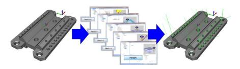
When the machining feature is ready there will be a "Finish" button that allows the operator to create the toolpath for the feature. Machining features can easily be edited by opening the wizard and making changes, then saving the new changes. When evaluating CAD/CAM, make sure the software supports the use of Wizards to program machining features.
