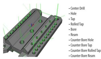
Some CAM systems will list them differently than others. Essentially, by navigating to the machine setup feature, you will have access to all of the 2, 3, 4 and 5 Axis machining strategies or features depending on the software.
