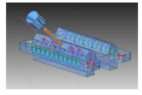
Some jobs require holes to be machined on angled surfaces where a 4th axis index is required. CAM software should allow the operator to set up an index system within a job if a 4th axis is required. This is where an output rotary angle would be used with and angle supplied by the operator. Here is an example where a 225 rotation angle and a 315 rotation angle were used in creating a program that had holes of various sizes on different planes.
